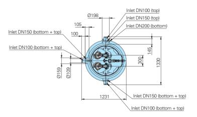
SK 9-40/1 Single pump station (dimensions same as twin pump station)
