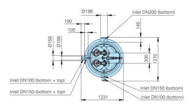
SK 6-40/1 Single pump station (dimensions same as twin pump station)
