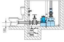
**Direct connection** Free standing WC (Inlet height 250 mm)
